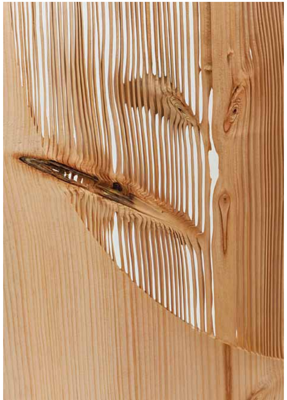
Right The sandblasting process leaves fine gaps between the wood's hard winter rings
